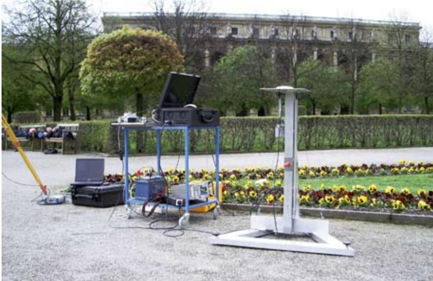
FIGURE 17 Lift for GPS receiver tests to simulate aircraft motion
